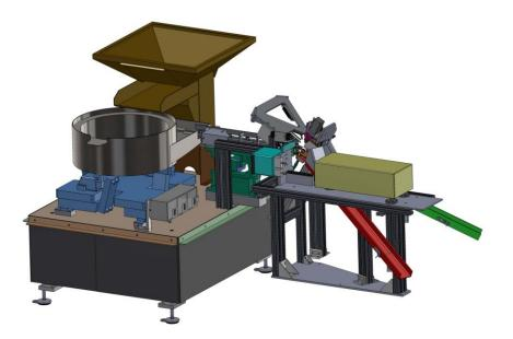
Figure 1: Machine designed to laser mark a cylindrically-shaped medical device at various locations
